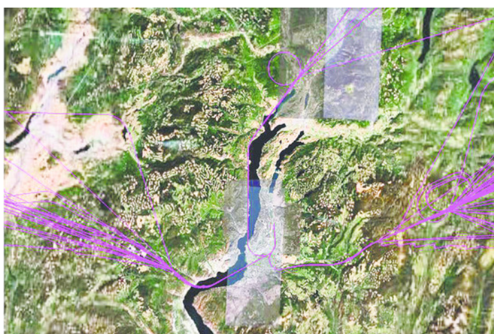
Radar tracks of WestJet Airlines after RNP procedures were activated show how the new system allows more-precise tracks for flights.
