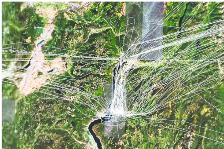
Radar tracks of WestJet Airlines flights at Kelowna, British Columbia, before RNP procedures were put in place.
