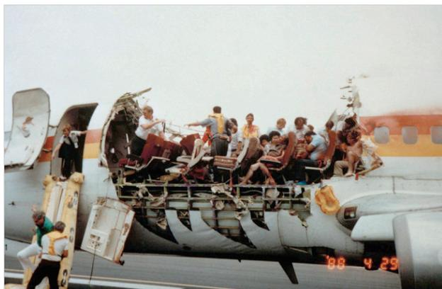
The cabin roof ripped off an Aloha Airlines 737 in 1988, having been weakened by metal fatigue. It is a recurring problem.
