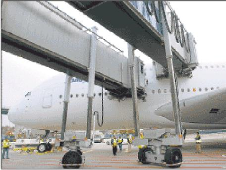
Passengers can board through two bridges—connected to the main level, or to main and upper levels—simultaneously. Typical boarding of 555 passengers could take more than 45 minutes.
