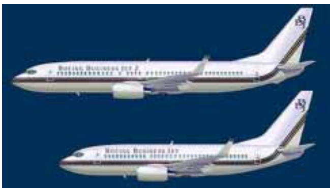
The Boeing Business Jet 2 (BBJ2) is a development of the BBJ family, with increased cabin volume and cargo volume.
