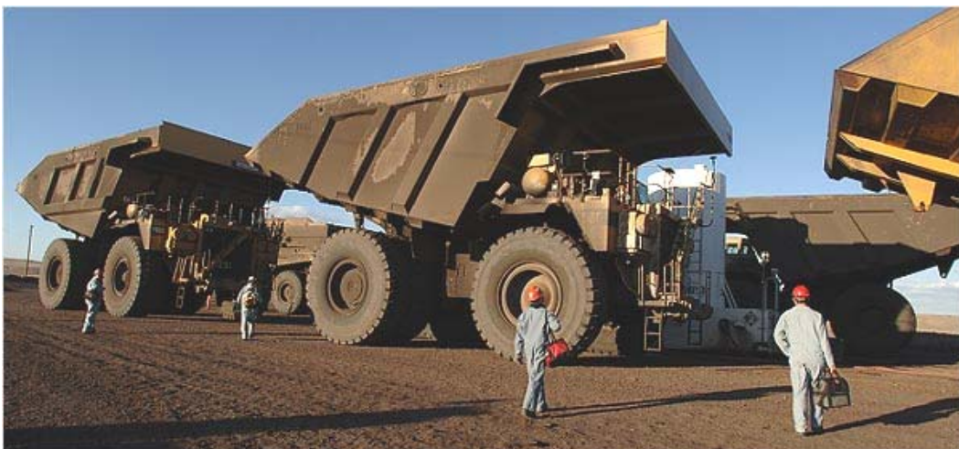
A mining truck that can carry as much as 400 tons of coal in Campbell County, Wyo. (関連記事 P-38)
